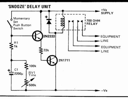
This unit is intended to turn off a piece of equipment after a predetermined time. The supply voltage is taken from the equipment to be switched and the relay contacts are wired in parallel with the power switch on the equipment.
